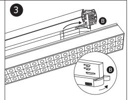
Rotate adaptor lock B clockwise 90° to connect the adaptor to the neutral circuit.
