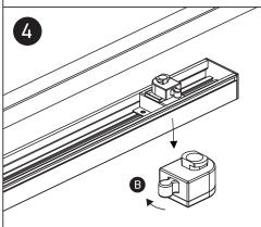
Rotate security button B anticlockwise 90° to secure track light to the track.
