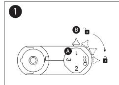
To mount the track adaptor into the track system, first check that the selector knob (A) is at OFF position and the adaptor lock **B** is disengaged.
