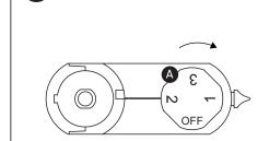
Circuit 1: Rotate the knob (A) 90° clockwise from the starting position OFF, to connect circuit 1.
