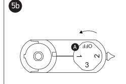
Circuit 2: Rotate the knob (A) 90° anti-clockwise from the starting position OFF, to connect circuit 2.
