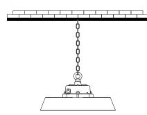
Use a chain, cable, mounting hook, or other mounting hardware to suspend the luminaire. Make sure the mounting hardware is securely attached to a stationary structure and strong enough to safely suspend the luminaire.
