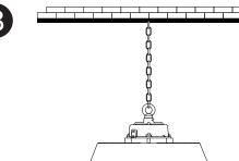
Use a chain, cable, mounting hook, or other mounting hardware to suspend the luminaire. Make sure the mounting hardware is securely attached to a stationary structure and strong enough to safely suspend the luminaire.
