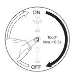
MEMORY OF BRIGHTNESS. Every time switch on the lamp, the lighting brightness is the same as the previous setting.
