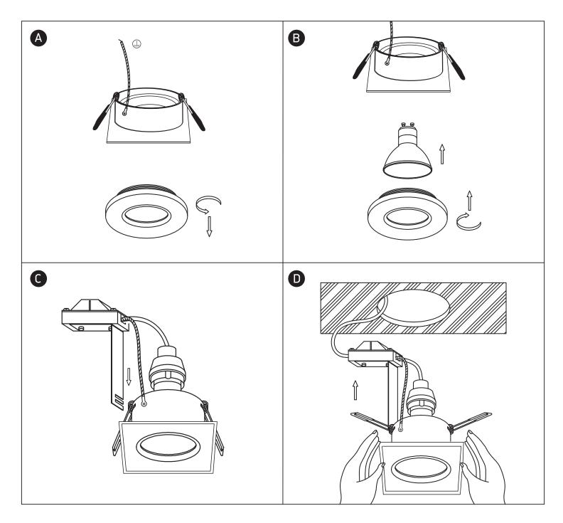
\*IP65 is the protection degree for the visible part of the fitting under the ceiling. The part of the fitting hidden in the ceiling is IP20.
