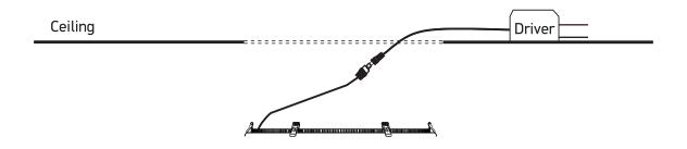
Install fitting using springs supplied.
