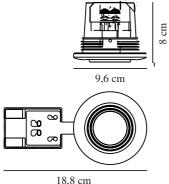
Voltage (V): 220-240 Volt IP degree: IP44 Maximum bulb wattage (W): 7,5W LED Class (Class 1, Class 2, Class 3): Class 2 (Double isolated) Socket type: GU10 Parallel connection: True
