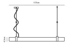
Voltage (V): 220-240 Volt IP degree: IP20 Class (Class 1, Class 2, Class 3): Class 2 (Double isolated) Bulb base: LED Module Dimmerable: True Switch placement: On the base Parallel connection: False
