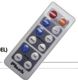
Infrared remote control for adjusting the movement and day light sensor parameters on the light fittings equipped with it. Parameters with which the luminaires are initially delivered are: 100% for the detection area, 50 lx for the daylight level and 1 min. the holding time.
